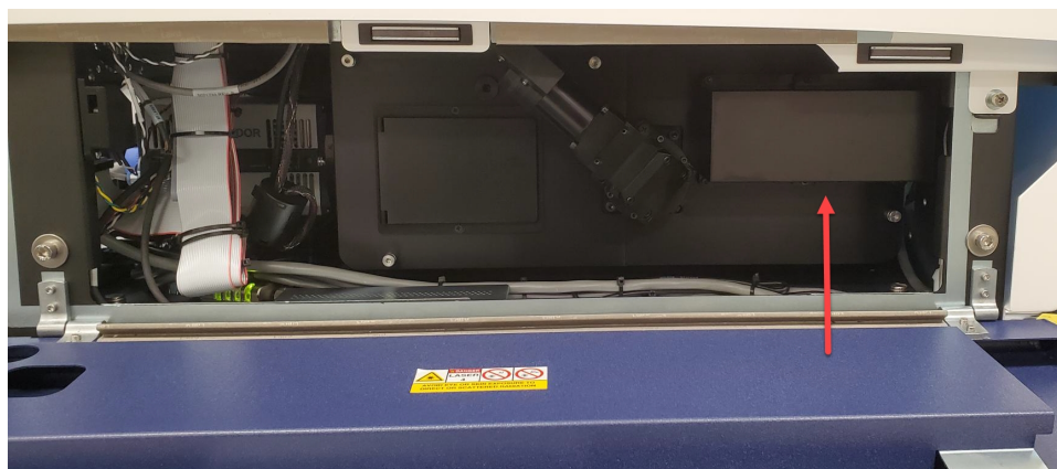
Figure 8-1: Disk Box Location in the Confocal Module Housing
