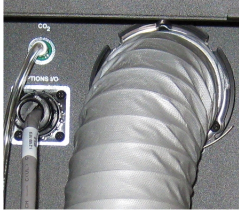
Figure 7-3: Warm Air Hose and CO 2 Tube on the Back of the ImageXpress Confocal HT.ai System
