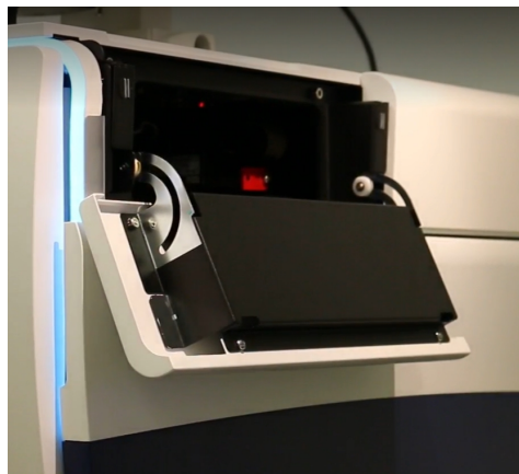
Figure 7-29: Right Side Upper Access Door
