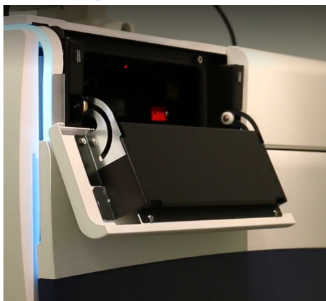
Figure 7-16: Right Side Upper Access Door
