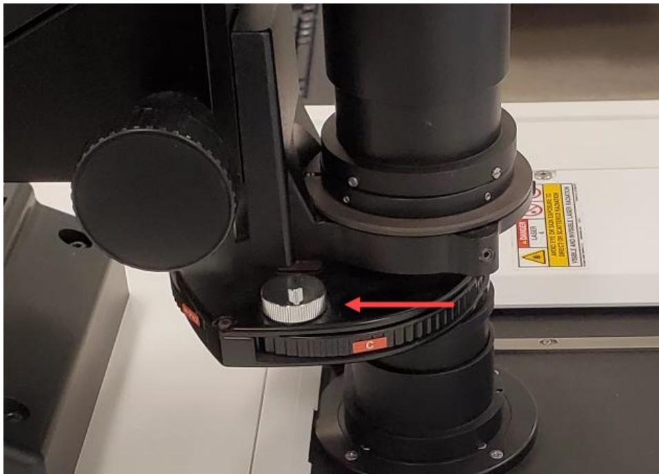
Figure 7-49: Centering the Condenser Annulus Ring with the Objective Phase Ring
