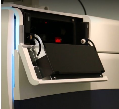
Figure 7-12: Right Side Upper Access Door
