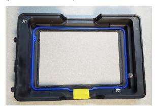
Under certain magnifications, a plate with a low skirt height may cause autofocus issues inside the environmental control cassette. The plate skirt height adapter sits inside the environmental control cassette to raise the plate, which can help autofocus succeed.
