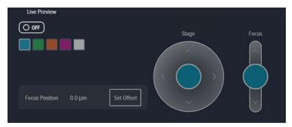
One joystick controls stage movement, allowing you to pan around the sample.
