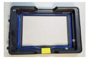
Under certain magnifications, a plate with a low skirt height may cause autofocus issues inside the environmental control cassette. The plate skirt height adapter sits inside the environmental control cassette to raise the plate, which can help autofocus succeed.
