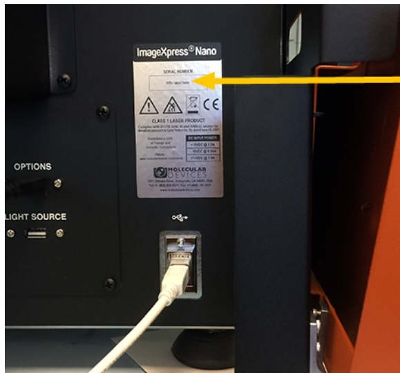
Figure 1-1: Serial Number location on the back of ImageXpress Nano
