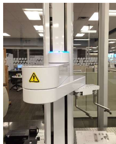
Figure 18 – SCARA in Safe Position and Orientation
