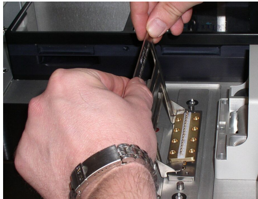
Figure 6-4 Removing the electrode base plate with the extraction tool.
