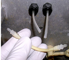
Figure 16-24: Removed Bad Tube Insert
