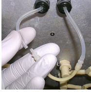
Figure 16-23: Separated Bad Tube Insert from 1/8" OD Tubing
