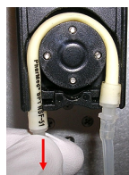
Figure 16-29: Pull Down Replacement Insert Tube to Position Clear 7/32" OD Tubing
