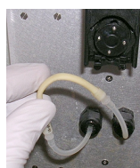
Figure 16-22: Tube Insert Removed from the Rotor Wheel
