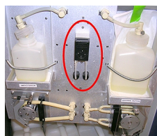
Figure 16-19: The Amphotericin Peristaltic Pump Within the Lower Compartment Fluid-Handling System
