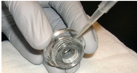
Figure 15-6: REGE Housing Threads Lubrication with 20 \mu l Distilled Water
