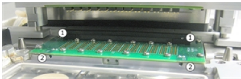
Figure 16-12: The Right Side PatchPlate Optical Sensors
