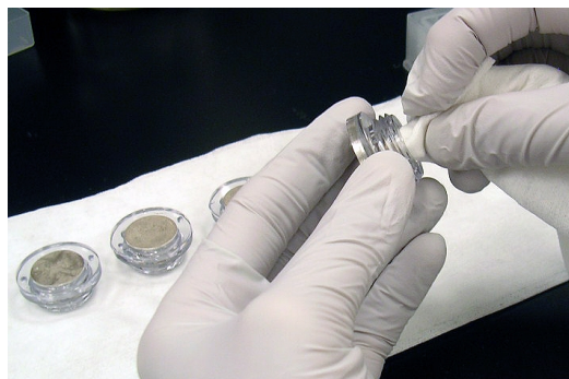
Figure 15-2: REGE Housing Underside Drying
