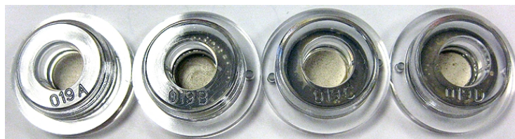
Figure 3-8: Serialized Set of Replaceable Ground Electrodes
