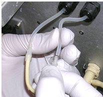
Figure 16-25: Attaching Replacement Insert Tube
