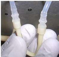
Figure 16-26: Completed Replacement Insert Tube Attachment
