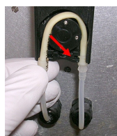
Figure 16-21: Stripping Tube Insert off of the Rotor Wheel
