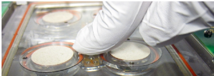
Figure 15-10: Gloved Finger Flush Installation Test
