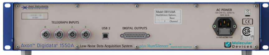
Figure 3-5: Rear panel of the Digidata 1550A digitizer.
