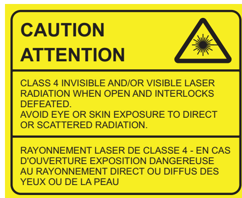
Figure S-4: Laser Label on the Bottom of the SpectraMax i3 Multi-Mode Detection Platform
