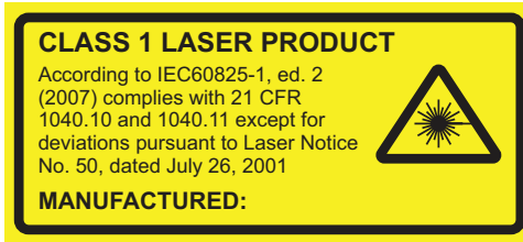
Figure S-2: Laser Label on the Rear of the SpectraMax i3 Multi-Mode Detection Platform
