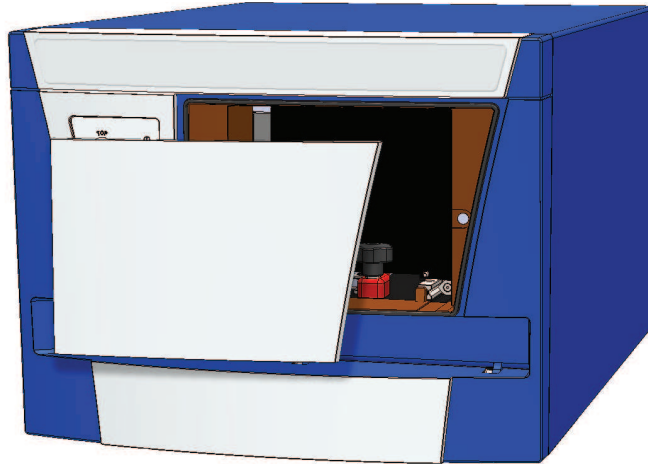
Figure 3-4: Detection Cartridge Drawer Cover Removed
