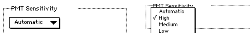
Figure 4.31: PMT Sensitivity Setting (SPECTRAmax GEMINI or GEMINI XS). Clicking in the box causes a menu of choices to appear. Automatic is present only when endpoint mode is chosen. Otherwise, settings are manual and limited to High, Medium, or Low.
