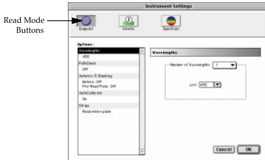
Figure 4.8: Instrument Settings for an Endpoint Reading. You can choose up to 6 wavelengths with SPECTRAmax or up to 2 wavelengths with VERSAmax instruments; choose 1 or 1-Ref with Emax, Vmax, UVmax, or THERMOmax instruments.
