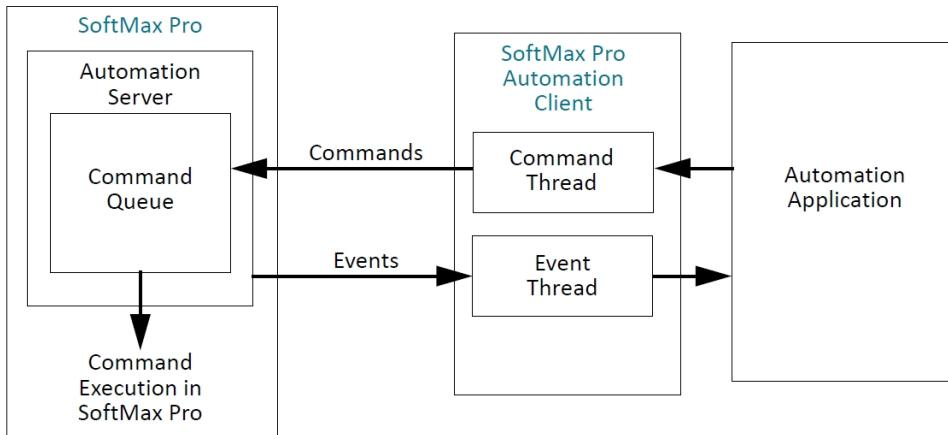
The .NET assembly SoftMax Pro Automation Client supplies the automation interface that controls the SoftMax Pro Software. This automation interface supports commands that trigger the event handlers to notify the automation interface application of the status of the SoftMax Pro Software, execute queued commands, and display errors. The applications you use to control the SoftMax Pro Software via the automation interface must connect through the Automation Client.
