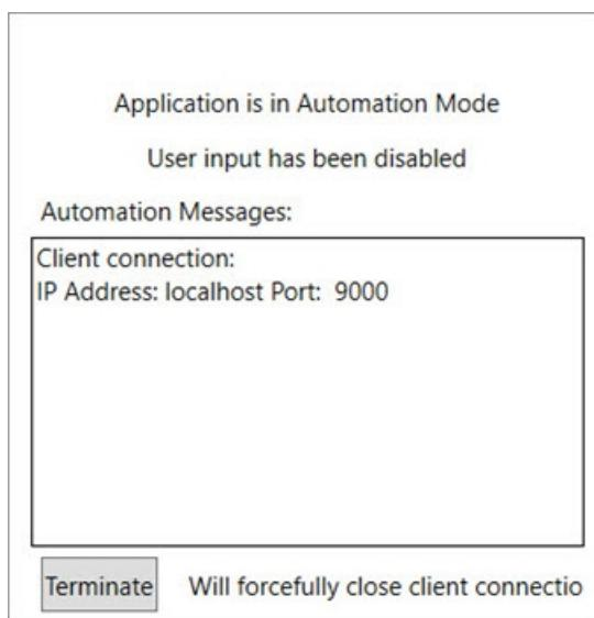
Click **Terminate** to stop the automation mode and regain control of the SoftMax Pro Software. Then close all open dialogs in the Excel workflow.
