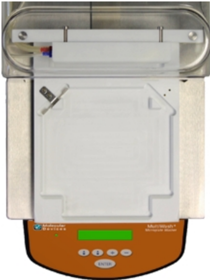
Figure Q-11: Installed Microplate Carrier
