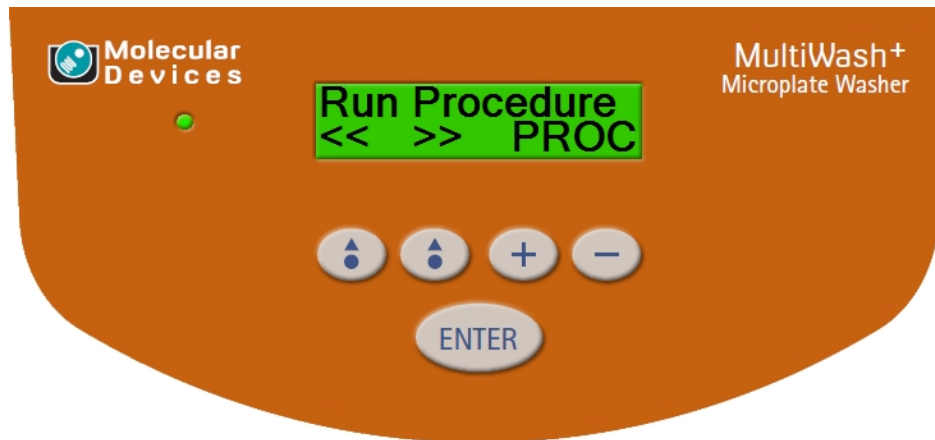
Figure 2-1: Instrument Control Panel
