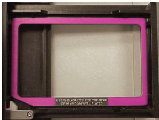
Figure 1.3: Microplate drawer (with adapter inserted).
