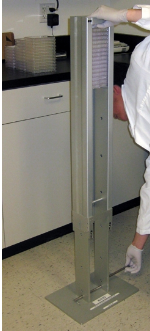
Hold Cassette and Move Support Pin
