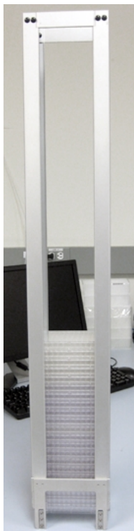
Stacker Cassette Bottom with Black Plate Holding Clips
