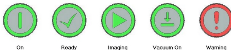
Figure 2-2: The functions of the indicator lights.
