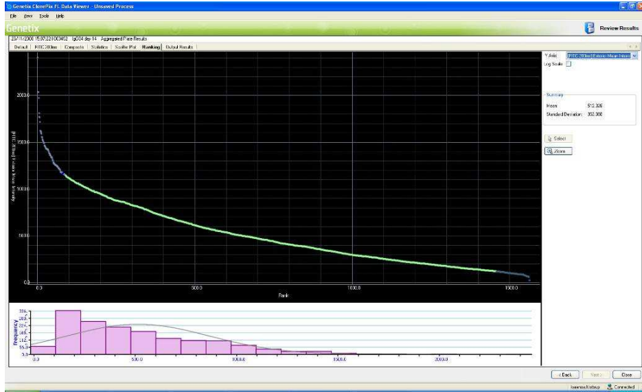
Figure 18: Rank Plot from ClonePix FL software showing the order of detected colonies from high to low fluorescence
