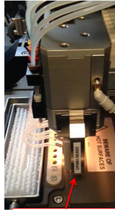
Halogen Drying Station
