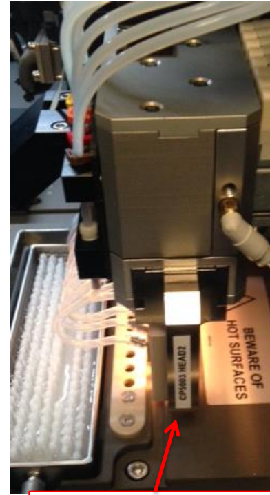
Halogen Drying Station
