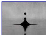
Figure 1. Stroboscopic image of 2.5 nL droplet ejection by ADE.
