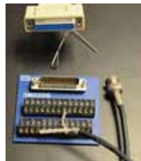
Fig. 1 One method to connect one line of a parallel port to equipment having a BNC connector. The end of a parallel cable (top) mates with the connector on the breakout board. A BNC connector-terminated coaxial cable has had one connector cut off. The signal wire is connected to pin 4 and the shield (ground) connected to pin 21. The BNC connector at the other end of the cable goes to the external control in of the device to be controlled.
