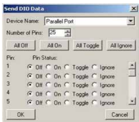
Fig. 4: Send DIO Data dialog. All pins of the Parallel Port device have been set off, i.e. low.
