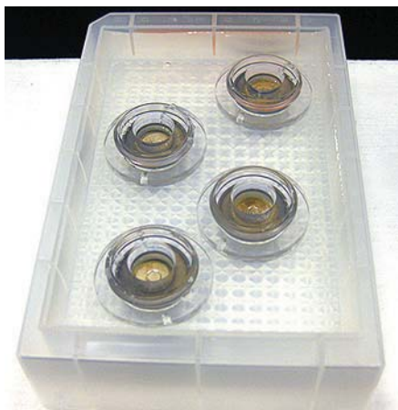
Figure 1-3: REGES Soaking in Condition Solution
