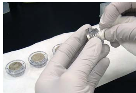
Figure 1-4: REGE Housing Underside Drying
