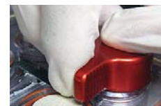
Figure 1-7: Two Hand Usage of the REGE Service Tool
