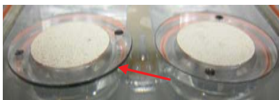
Figure 1-10: Incorrect Raised REGE Installation
