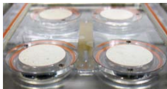
Figure 1-9: Correct Flush REGE Installation
