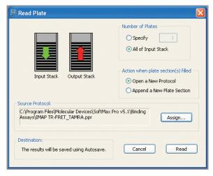
SpectraMax Absorbance, Fluorescence, Luminescence, and Multi-Mode Readers can be integrated with the StakMax® Microplate Stacker. System setup and calibration are controlled from within SoftMax Pro 6 Software.
