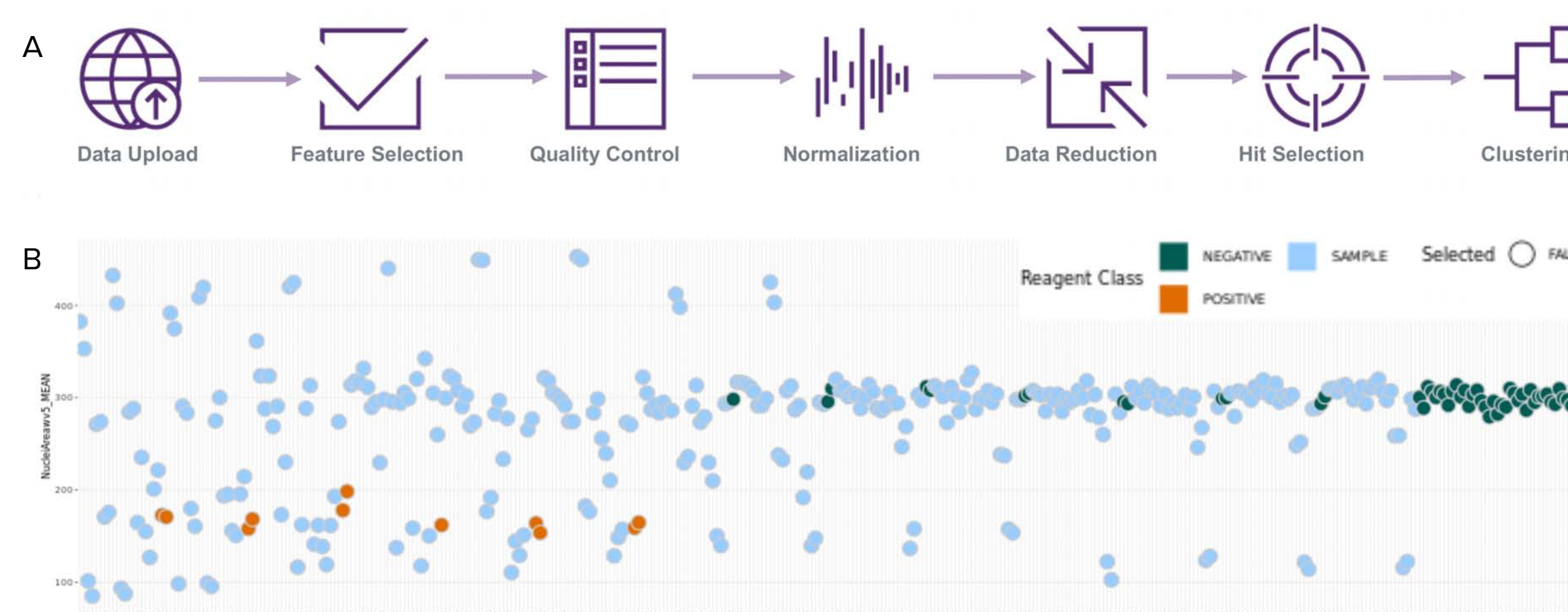
Figure 3A–B. Using HC StratoMineR for data analysis. A) HC StratoMineR is a web-based platform which guides users through a typical workflow in analysis of high-content multi-parametric data. B) Scatter plot from the QC step. The x-axis represents all samples, y-axis represents the selected feature (nuclei area).
